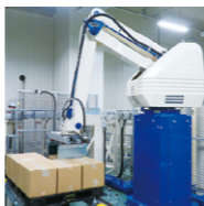
Introduced a robotic de-vanning and palletizing system (DPS)
